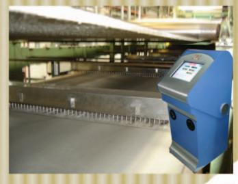
THERMOCON was built on the success of our Model EZC-1 Zero Crush Bar. The same patented technology was applied to THERMOCON to achieve unprecedented accuracy in pressure control on the corrugator hotplates.
